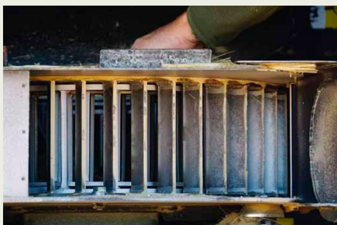
The cage mill pulverises 95 per cent of weed seeds into unviable chaff (photo: Glyn Jones, ABC Landline)
